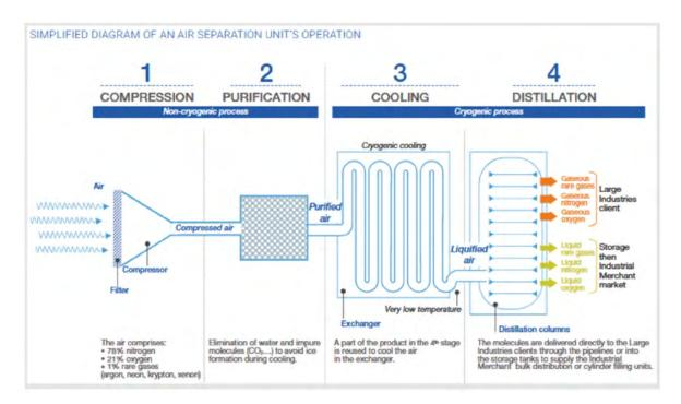
Used in a wide variety of fields, large air separation units (ASU) produce high purity oxygen, nitrogen, argon and rare gases through a combination of adsorption purification, cryogenic distillation and internal compression of high pressure product
