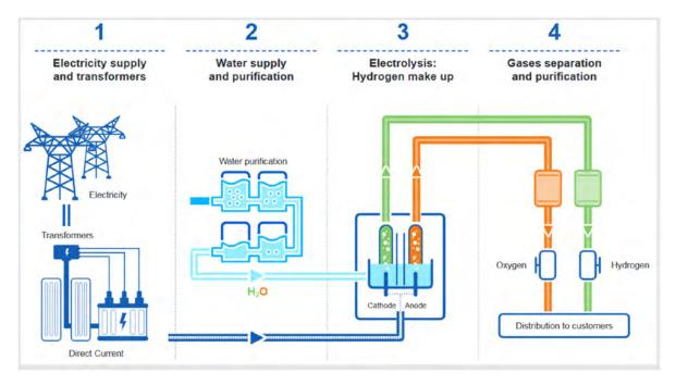
Hydrogen production through electrolysis is based on the dissociation of water molecules  $(H_2O)$  using electricity, to extract hydrogen and oxygen molecules. This process produces hydrogen without using or emitting carbon-based molecules. It can be used to produce carbon-free hydrogen for industry and mobility, as well as for electricity storage.
